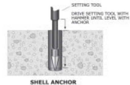
Figure 132: Set shell anchors.
